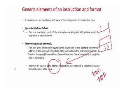
So, whenever I told that zero address means is nothing to be surprised; that means, in the instruction itself you are not saying where are the operands, but the there is a different stack attached to it and it will start operating on the elements of this stack my first pushing means popping them up and doing the operation and push back.
